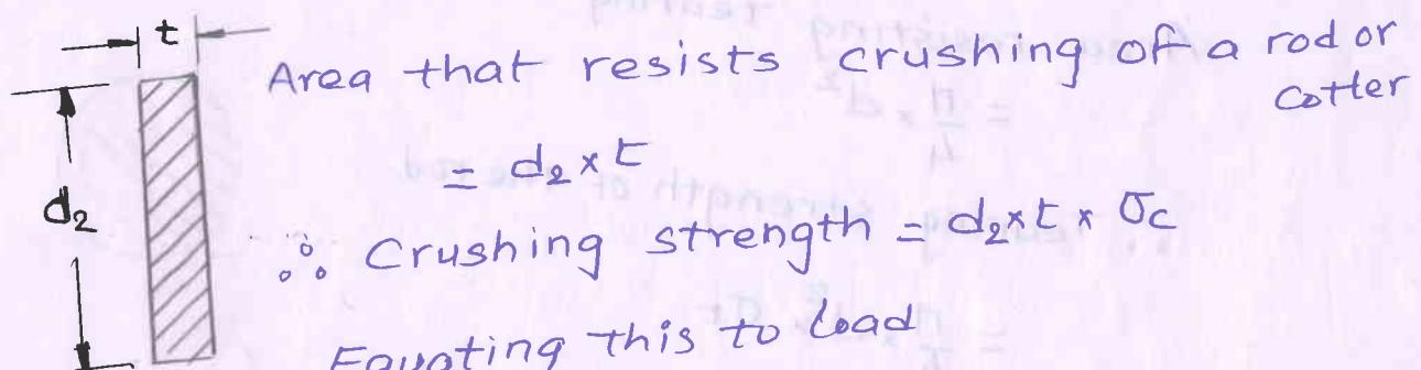
$$\therefore \text{Crushing strength} = d_2 \times t \times \sigma_c$$
