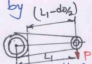
→ The bending stress corresponding to Max. bending moment in lever cross-section
