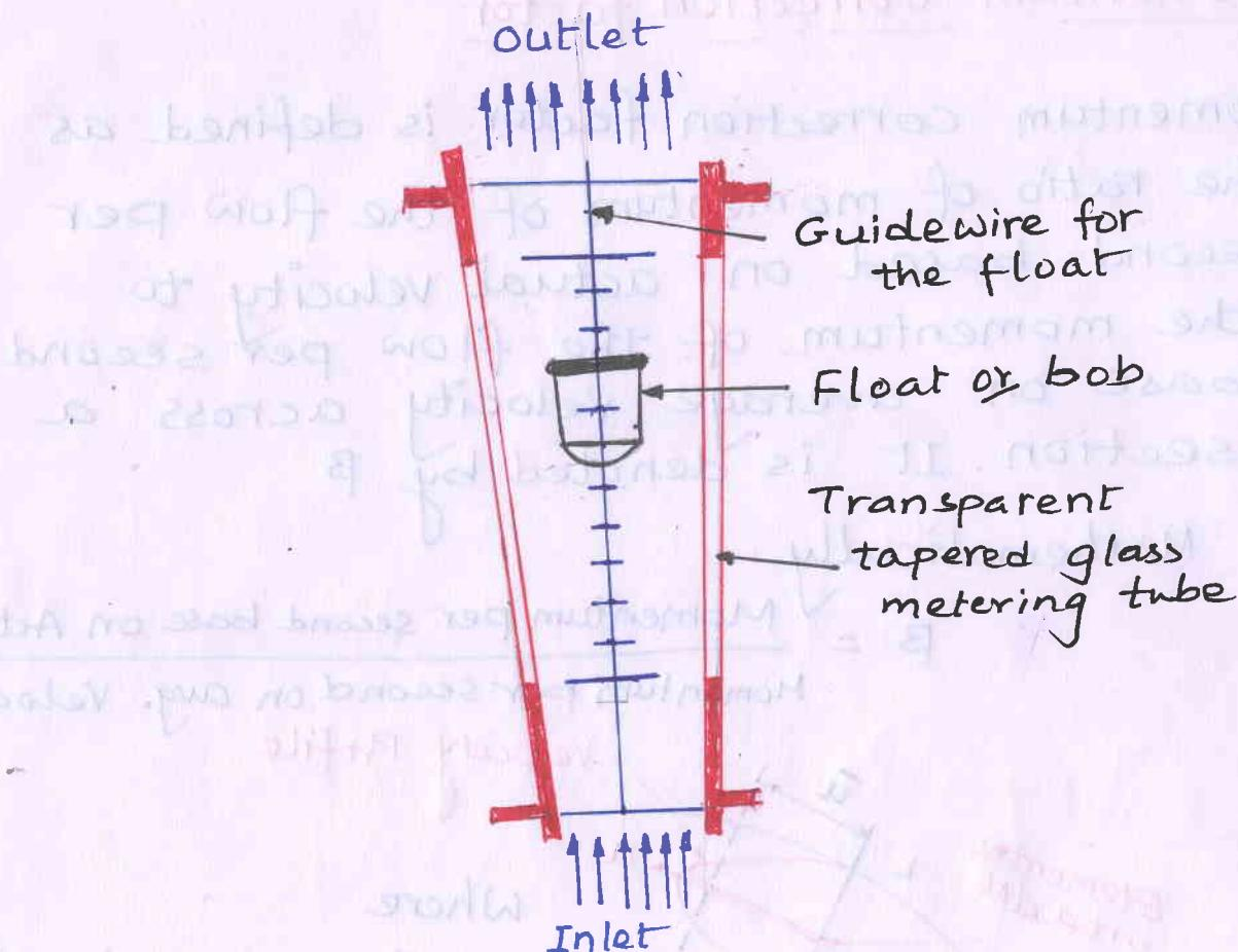
Working :- When the rate of flow increases the float rises in the tube and consequently there is an increase in the annular area between the float and the tube. Thus the float rides higher or lower depending on the rate of flow
