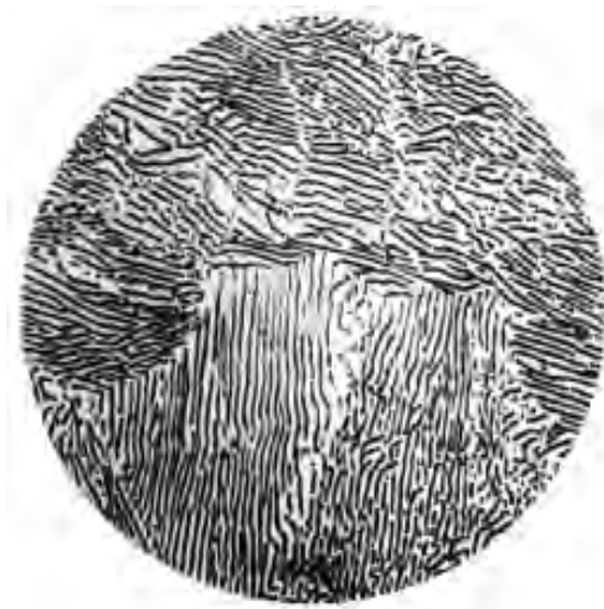
Figure 4.2 Microstructure showing lamellar nature of pearlite ( \times 1200 ).
