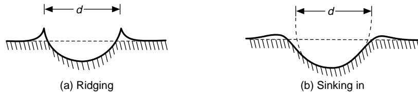
Figure 18.3 Localized deformation in Brinell testing.
