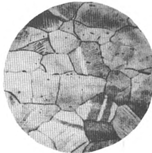
Figure 14.1 Microstructure of as-quenched Hadfield steel (1.4% C and 14.2% Mn) showing austenitic grains; water quenched from 1050°C (×100).
