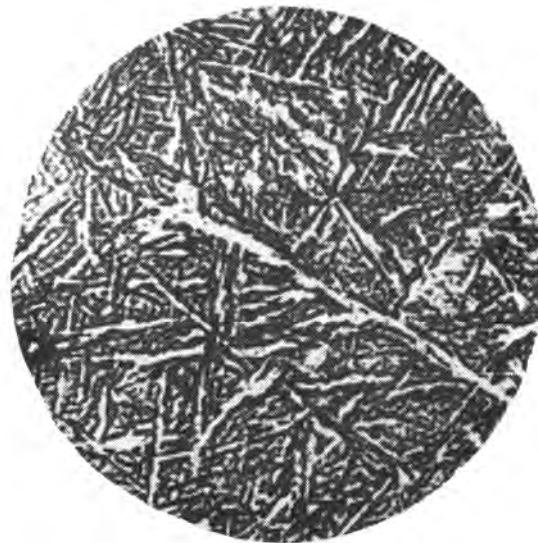
Figure 5.6 Microstructure showing coarse accicular martensite ( \times 300 ).
