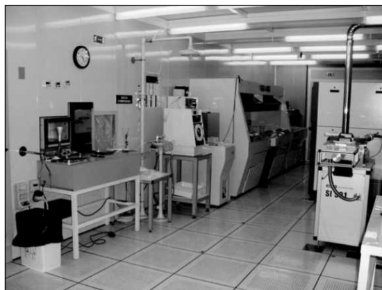
Fig. 20.5 A clean room for lithography usually hosts a self-contained infrastructure. Commonly seen facilities are spin-coater, mask aligner, photolithography stage, lamellar chemical hood, physical vapor deposition unit, microscopes, etc. (reproduced from ref. 7). (For clarity see colour figure.)
