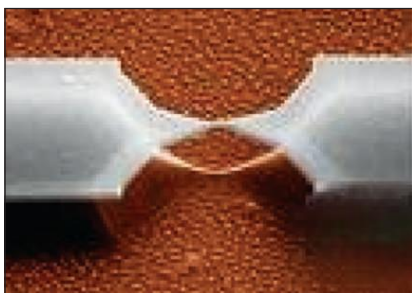
Fig. 19.2 Break-junction setup: a very narrow contact is stretched by flexing the support until single atom makes the contact (adapted from a website (ref. 7)).
