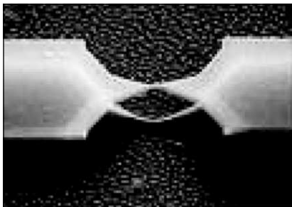
Fig. 19.2 Break-junction setup: a very narrow contact is stretched by flexing the support until single atom makes the contact (adapted from a website (ref. 7)). (For clarity see colour figure.)
