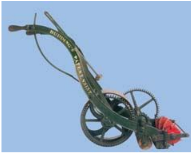
Lawn-mover is a combination of kinematic links.
