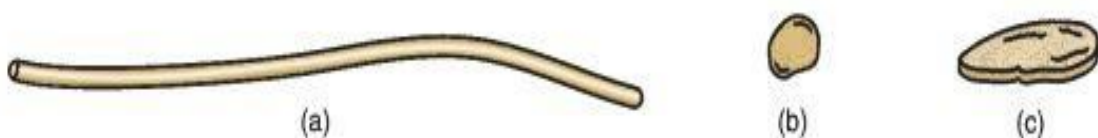
Fig.4.2 Possible physical shapes of imbedded phases in composite materials: (a) fiber, (b) particle (c) flake.
