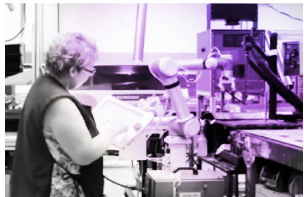
Operator programming a cobot on wheels for line discharge
