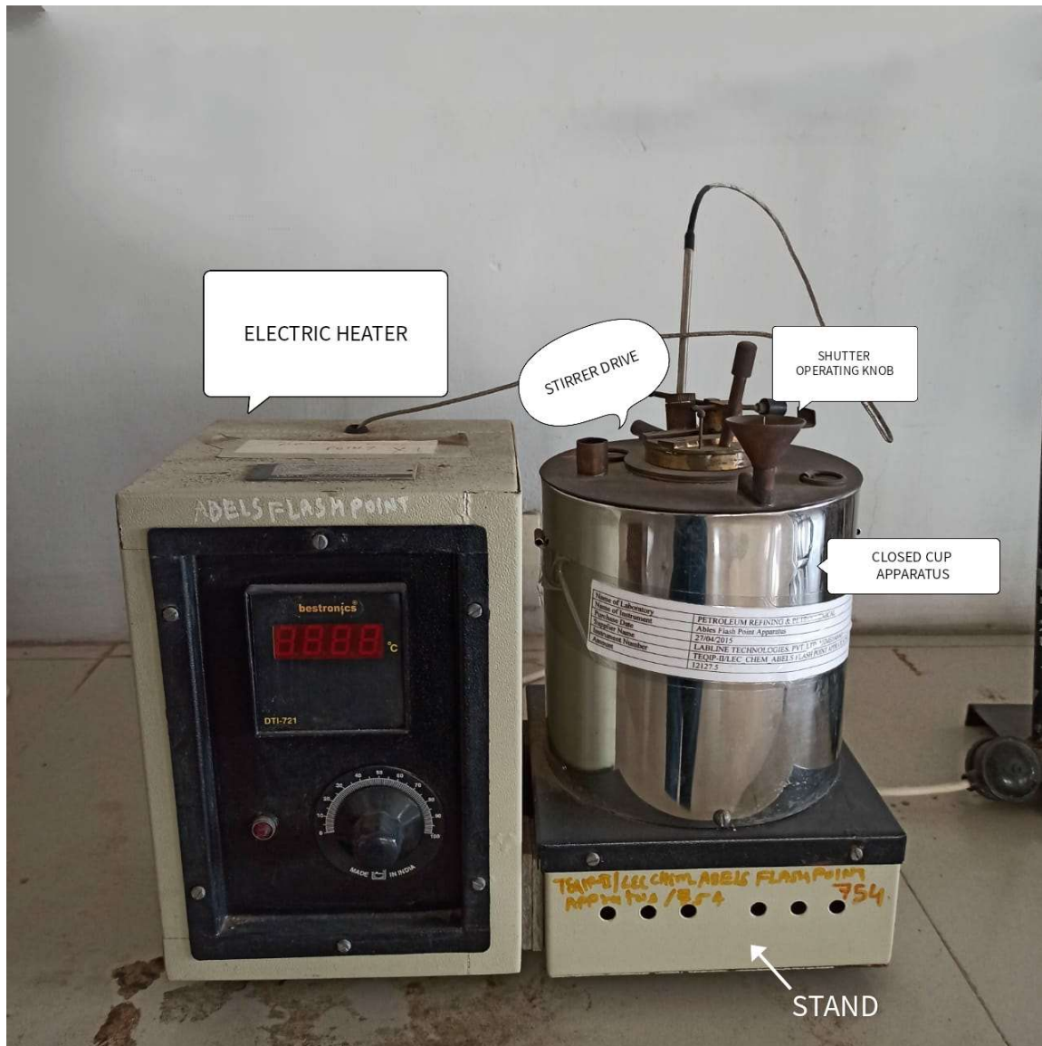
Abel's Flash Point Apparatus: Assembly plus heating Vessel
