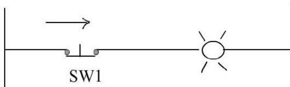
Hardwire switch-lamp circuit
