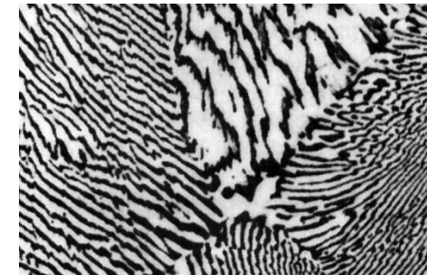
Micrograph of Pb-Sn eutectic microstructure
