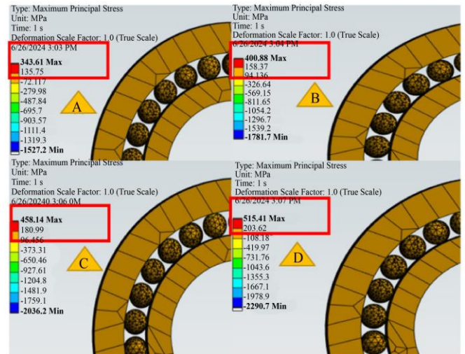
Fig. 12 Maximum principal stress result at various pressure magnitudes 60Mpa, 70Mpa, 80Mpa, 90 Mpa
