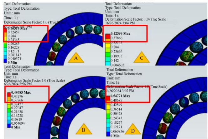
Fig. 11 Deformation results at various pressure magnitudes at 60Mpa,70Mpa,80Mpa, and 90 Mpa
